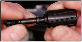
Step 6: Put some Blue 242 Loctite on the Threads of the Bolt.
